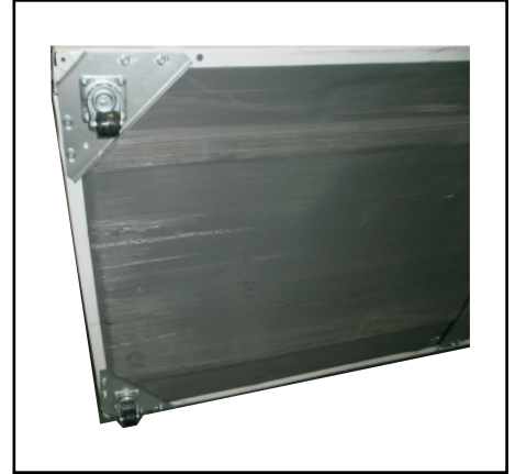
6. Casters are installed
