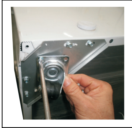
5. Fix the casters by screwdriver.
